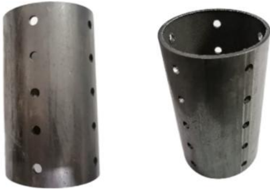
Figure 2: The perforated test specimen
