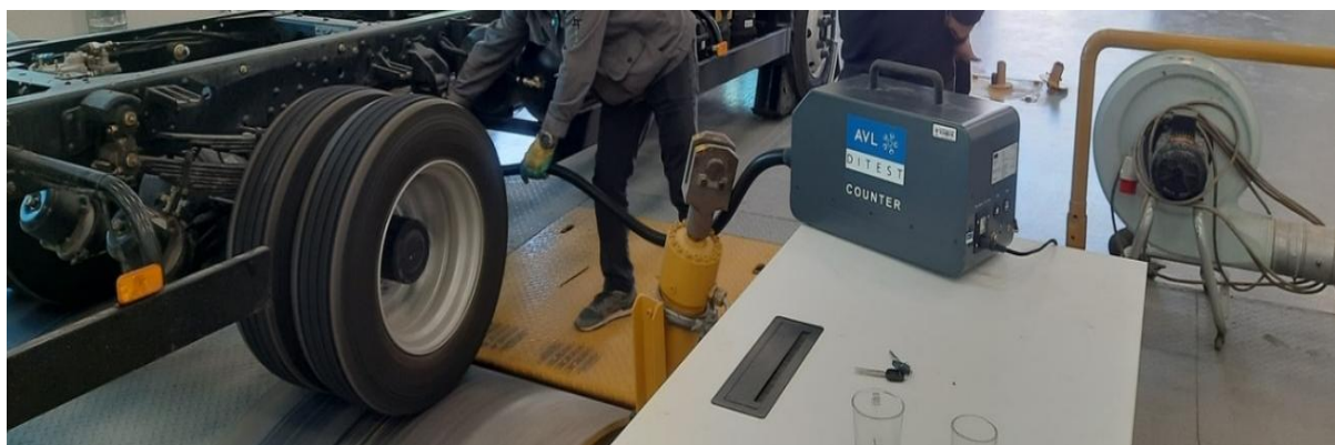
Figure 3: Device for measuring emitted particulate matter
