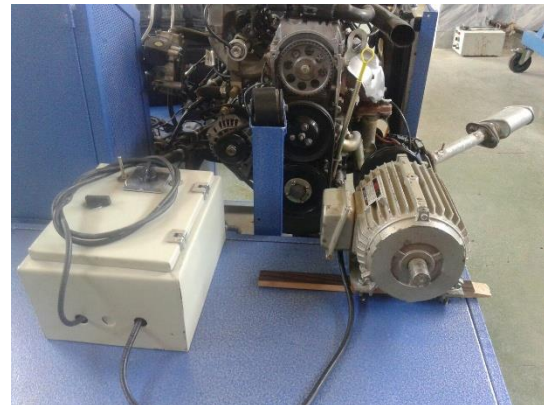
Figure 1: Motor setup, electric motor and inverter
