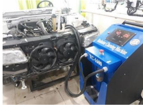
Figure 9: Radiator washing device connected to the water path between the engine and the radiator.
