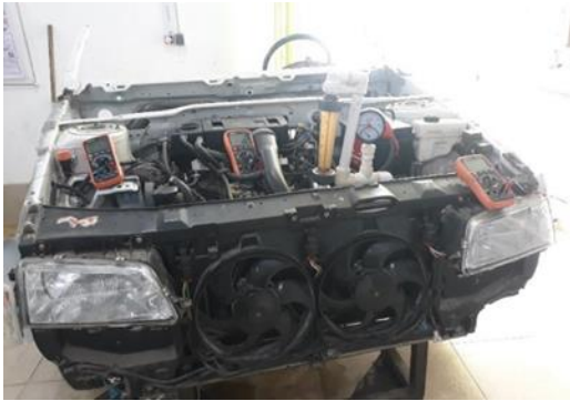
Figure 8: Measuring equipment installed on the XU7 engine
