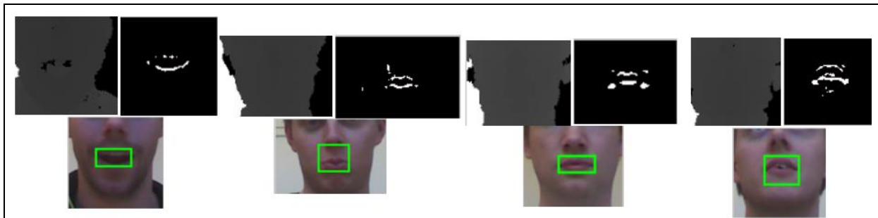
Figure6: Results of detecting closed mouths (second row) by applying the adaptive mask on the depth image (first row) for 4 different individuals.
